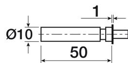
*Smove to decelerate the closure of the door. Make a Ø10 hole and insert the smove at the centre of the top or the base panel of the cabinet. For wood-based and alu-framed doors over 1.600mm height, it may be necessary to use two smove, one to be inserted into the top and the second into the base panel of the cabinet.*
